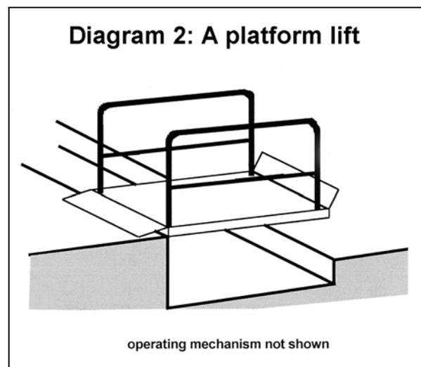
Platform lifts can also be sited in an external lift shaft attached to the building. Some installations can allow entry from opposite sides at different levels. A liftway enclosure should be provided where vertical travel is greater than 2m. Useful features of a platform lift are that, in general, only a very shallow pit is needed in the floor beneath the lift rather than the deep pit needed for a passenger car lift, and no motor room is required.
